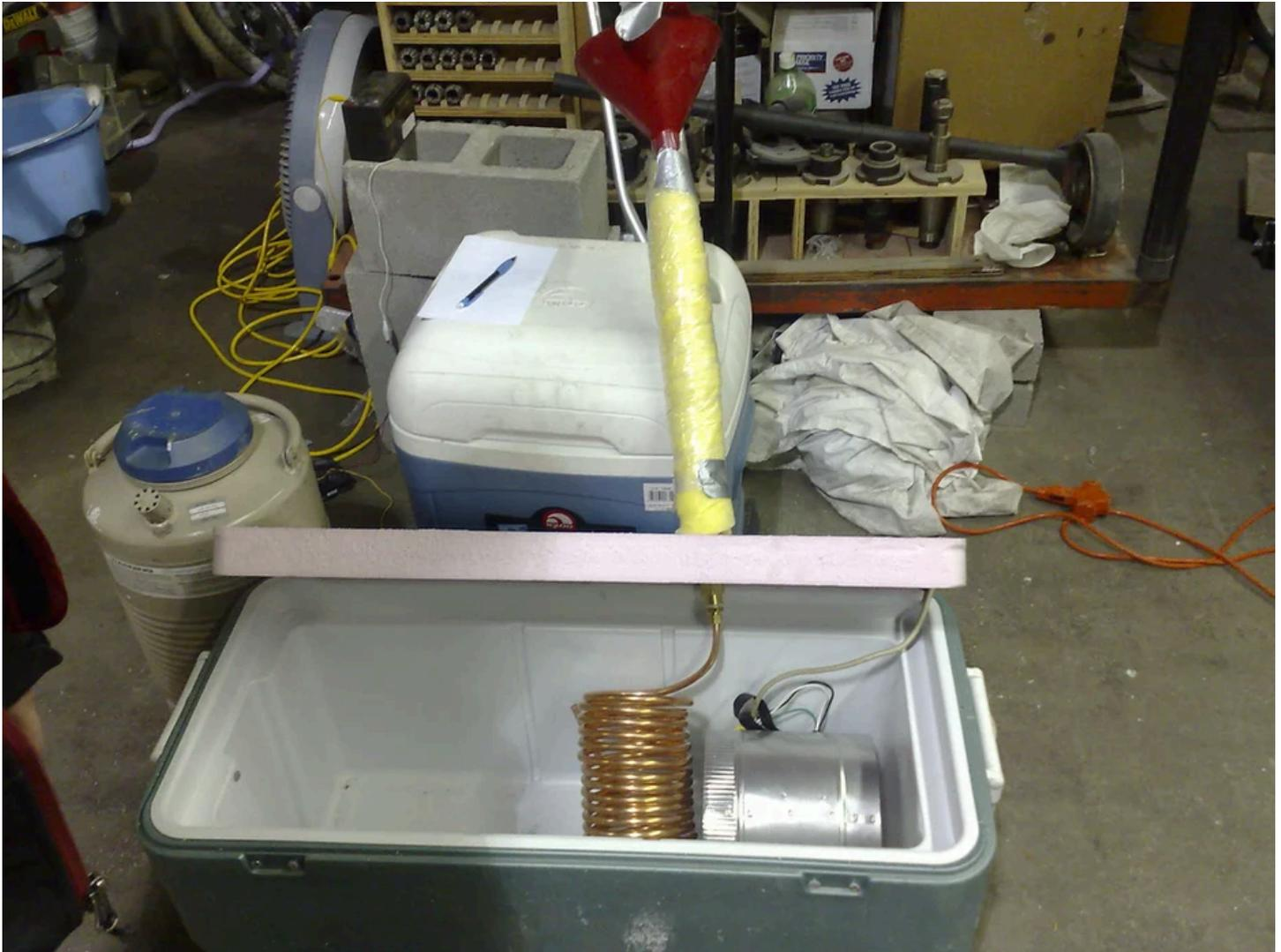
Getting stuff \*really\* cold is difficult, dangerous, and lots of fun. Our group is preparing to send an autonomous glider up to about 100,000 feet, so we needed a way to chill our electronics to  $-70^{\circ}\text{C}$  to test their use before these edge-of-space flights.
